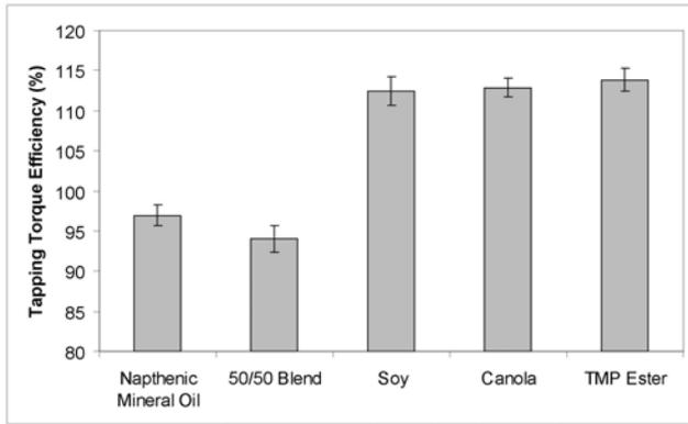
**Figure 3. Tapping torque efficiency for five different base oils (napthenic mineral, napthenic/paraffinic blend, canola, soybean, and TMP ester) as straight oils (100% wt).**
