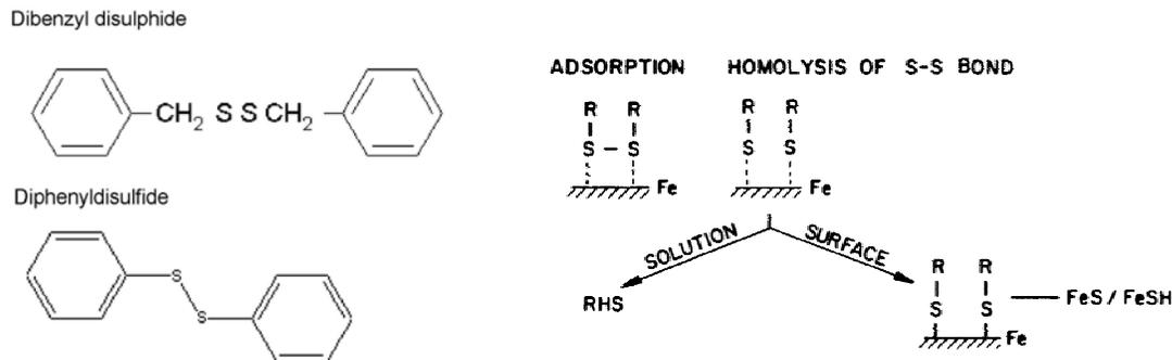
**Figure 7. (Left) Two candidate organo-sulfur EP additives for MWFs: dibenzyl disulfide and diphenyldisulfide. (Right) Proposed mechanism of organo-sulfur action in metal cutting after Bushan (1999) [11].**
