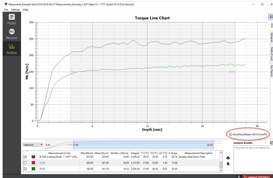
The function-button (On/Off) in the register „Graph“ provides a fast switch of the depiction to the unsmoothed raw data (Graph Smoothing).
