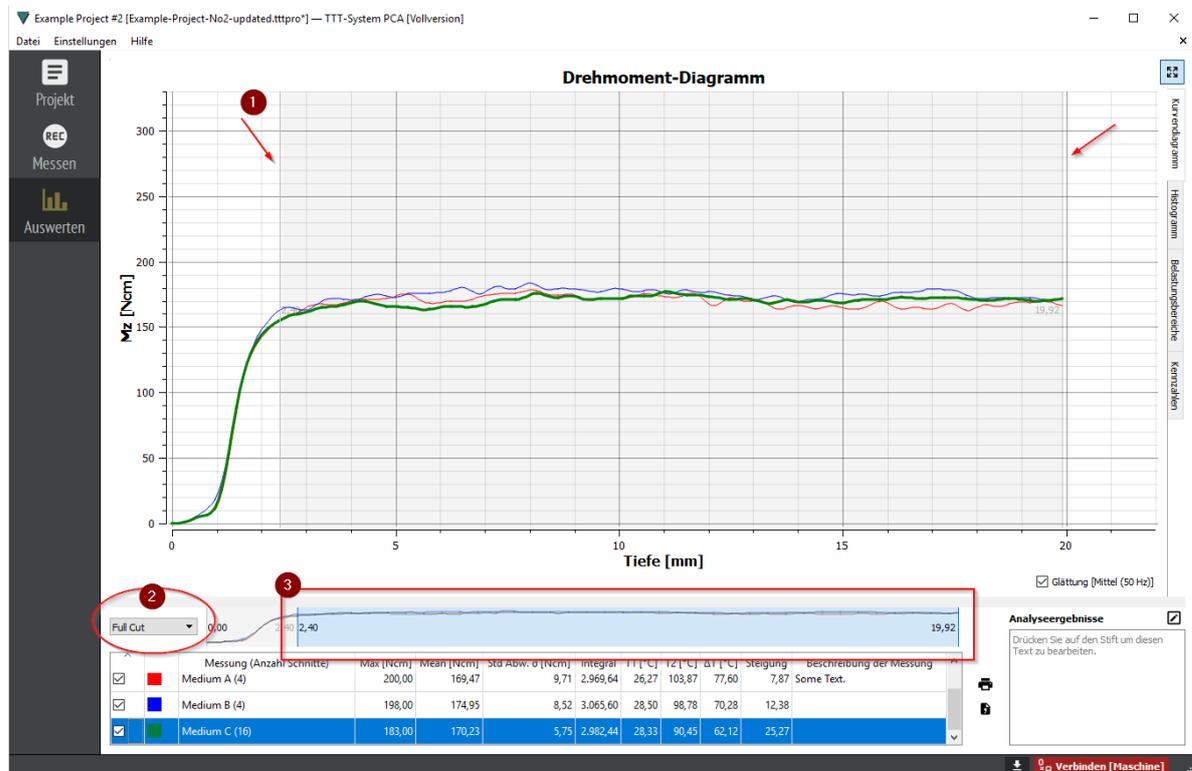
In the graph, the current segment is highlighted in gray (red arrows 1). It can be changed left and right at the edges of the blue segment display below the graph (red rectangle 3). On the left side of the segment representation the active segment is visible which can be changed there (drop-down menu under 2). **All data of the table or the key figure are ALWAYS valid only for the current segment** (this is not true for the temperature  $\Delta T$ ).
