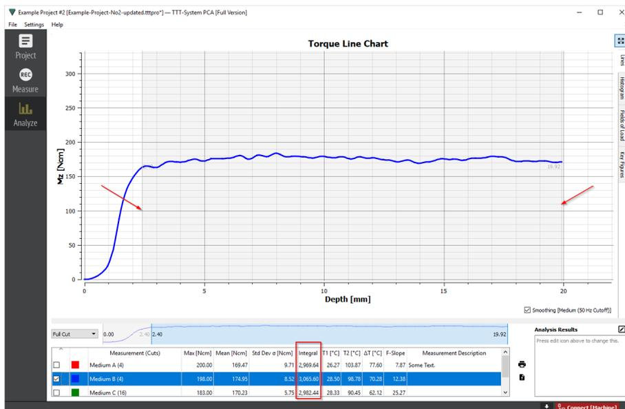
Integral as a value for the total stress (friction) on the measurement tool
