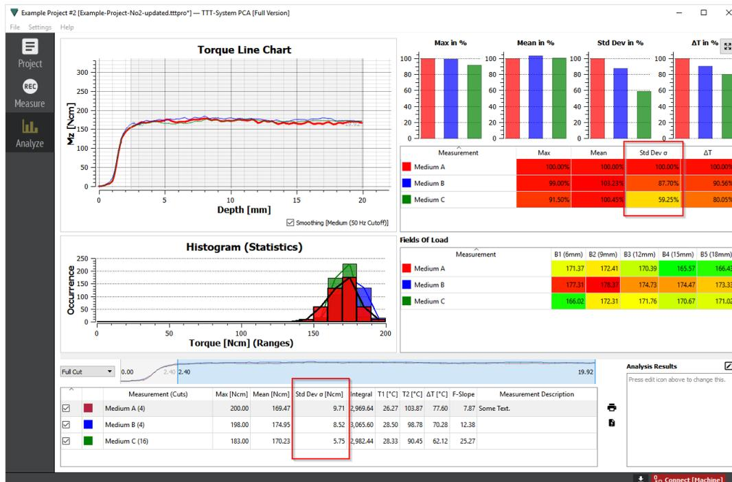
**Standard Deviation** as a value for the mean deviation of the torque around the Mean Value
