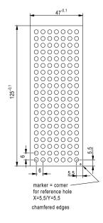
Every test-bar is manually gauged with tolerence 0,01 mm hole diameter. We deliver our test-bars with max. 6 bad holes, wich are red signed and identified.
