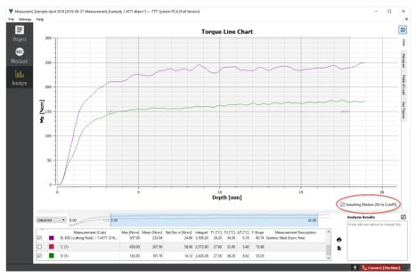
The function-button (On/Off) in the register "Graph" provides a fast switch of the depiction to the unsmoothed raw data (Graph Smoothing).
