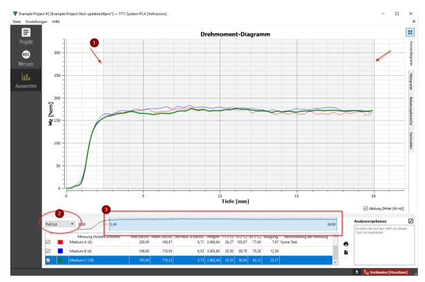
In the graph, the current segment is highlighted in gray (red arrows ①). It can be changed left and right at the edges of the blue segment display below the graph (red rectangle ③). On the left side of the segment representation the active segment is visible which can be changed there (drop-down menu under ②). **All data of the table or the key figure are ALWAYS valid only for the current segment** (this is not true for the temperature  $\Delta$ T).
