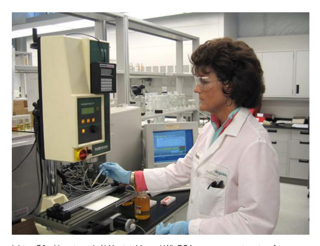
labtap G8 with automatic X-Yautotable and WinPCA measurement-system from microtap GmbH www.microtap.de
