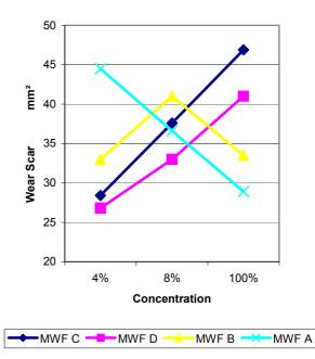
Figure 17: Reichert Al roll wear depending on MWF-concentration
