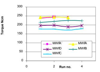
Figure 12: Thread Forming Al Mg Si0.5, MWF-conc. 8 %
