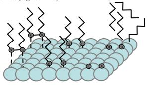
Physisorption Chemisorption Reaction Figure 2: Theoretical model of interaction between sulphur-carrier and metallic surface (5)[1]
