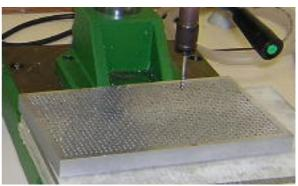
Figure 10: Microtap-testing plate
