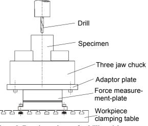
Figure 8: Experimental setup for drilling trial
