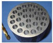
Figure 6: Specimen 16 Mn Cr5/drill
