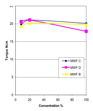
Figure 13: Thread cutting in 16 Mn Cr5
