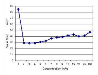
Figure 18: Reichert Al rolls activation concentration MWF C
