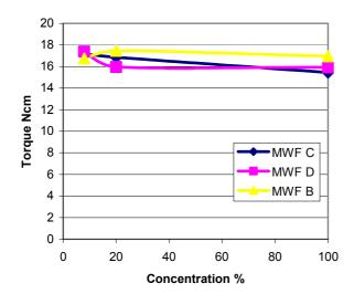
Figure 14: Thread cutting in GGG 60
