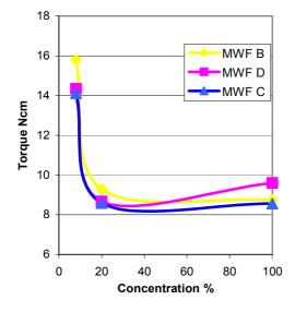
Figure 11: Thread cutting in Al Si18
