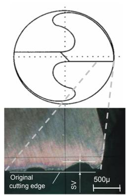
Figure 7: Cutting edge wear SV
