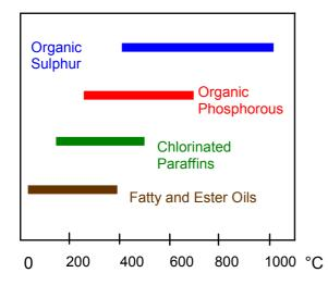
Figure 3: Activation temperature range of different lubrication additives
