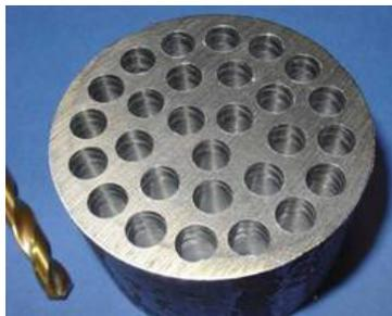
Figure 6: Specimen 16 Mn Cr5/drill
