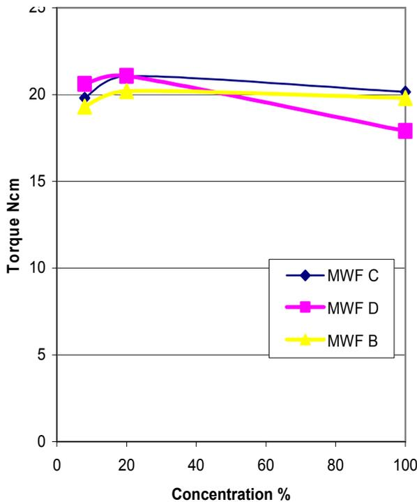
Figure 13: Thread cutting in 16 Mn Cr5
