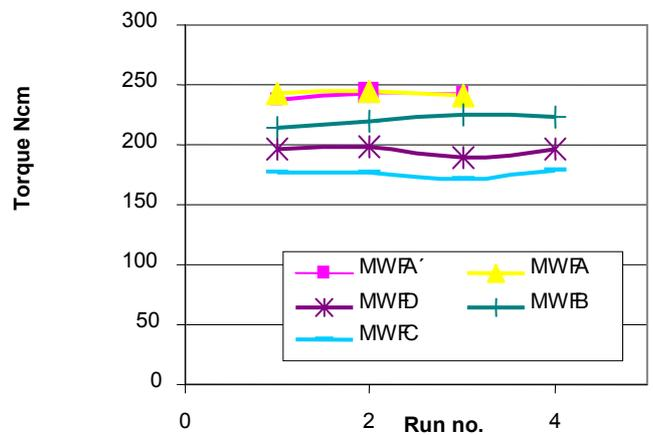
Figure 12: Thread Forming Al Mg Si0.5, MWF-conc. 8 %
