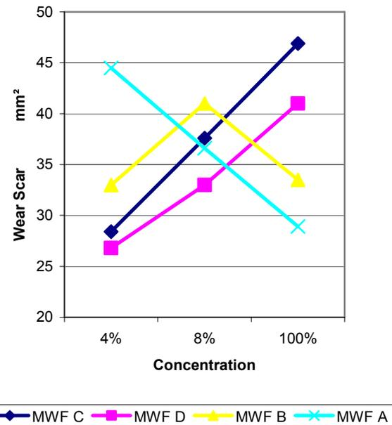
Figure 17: Reichert Al roll wear depending on MWF-concentration
