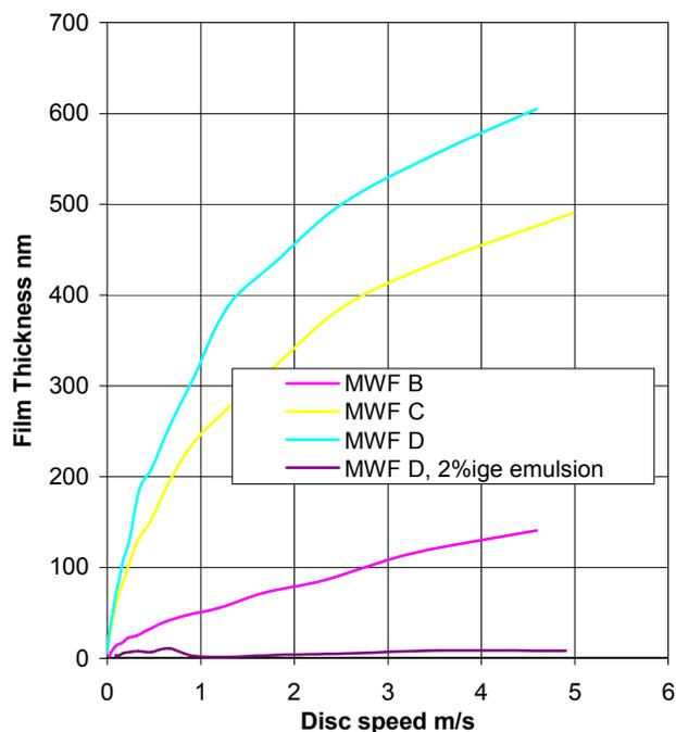
Figure 24: Optical Rig - Comparison film thickness concentrate/emulsion
