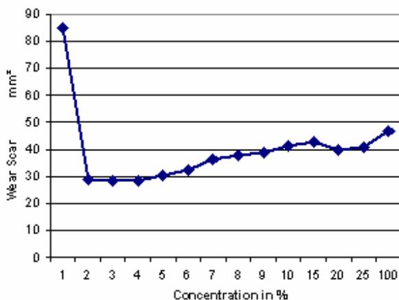
Figure 18: Reichert Al rolls activation concentration MWF C
