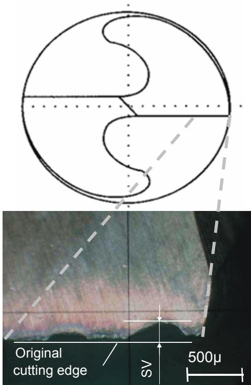
Figure 7: Cutting edge wear SV
