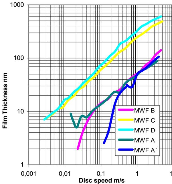
Figure 25: Optical Rig - Comparison of film thickness of different concentrates
